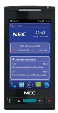
The SmartDECT handset G966 is a sophisticated handset providing enterprise grade capabilities and proven DECT voice quality with the flexibility of android application support.
