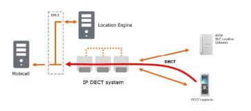
initiated by NEC DECT handsets such as the G577 and I766. In the background the BLE beacon ID of these handsets are detected in real-time by the Location Gateways and stored in the Location Engine. In this way entries and exits are guarded and records of devices passing through these doorways are stored.
