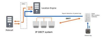
Mobicall will then follow up with the appropriate action like for instance locking the door, depending on preconfigured policies.
